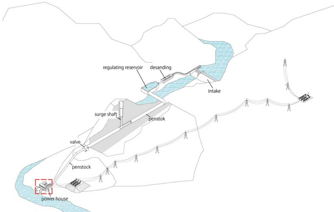
Figure 1: Layout of the hydro-electric installation
